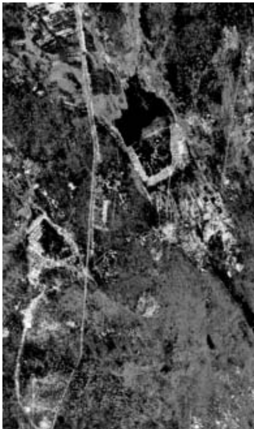
A spaceborne radar image of the Great Wall of China in a desert region about 400 miles west of Beijing. The wall is easily detected from space by radar because its steep, smooth sides provide a prominent surface for reflection of the radar beam. The image was acquired by the Spaceborne Imaging Radar-C/X-Band Synthetic Aperture Radar (SIR-C/X-SAR) aboard the Shuttle Endeavour on 10 April 1994. NASA Image 96-HC-228.
