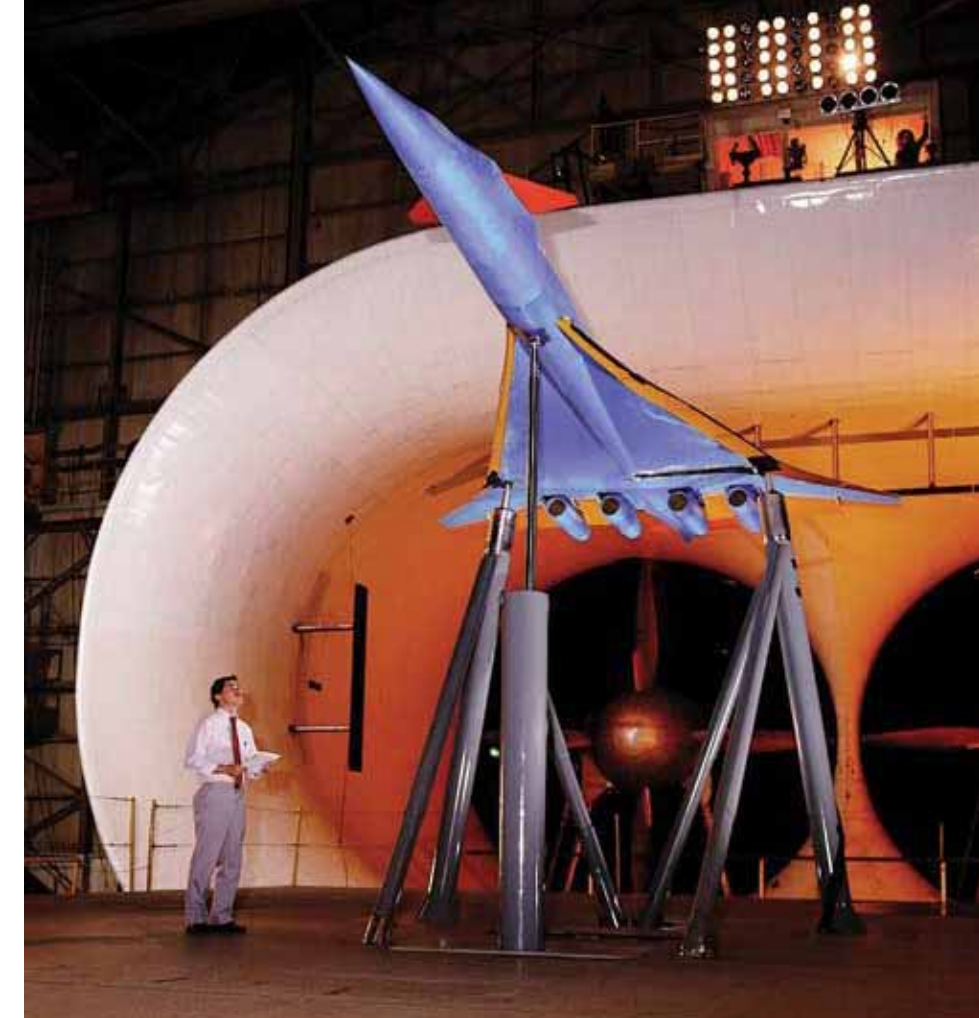
Researcher David E. Hahne inspects a 1/10-scale model of a McDonnell Douglas Mach 2.2 transport in the Full-Scale Tunnel in 1992.
