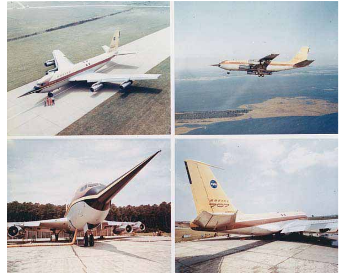
Boeing’s 367-80 was used at Langley for in-flight simulator studies of handling qualities of supersonic Transport configurations.
