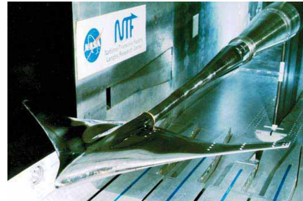
Blended Wing Body model undergoing tests in the Langley National Transonic Facility.
