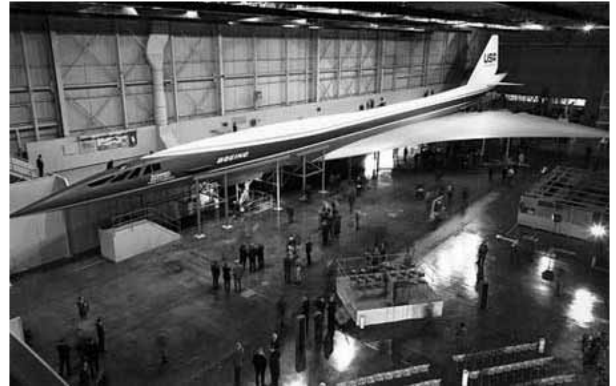
Engineering mock-up of the Boeing 2707-300 Supersonic Transport.
