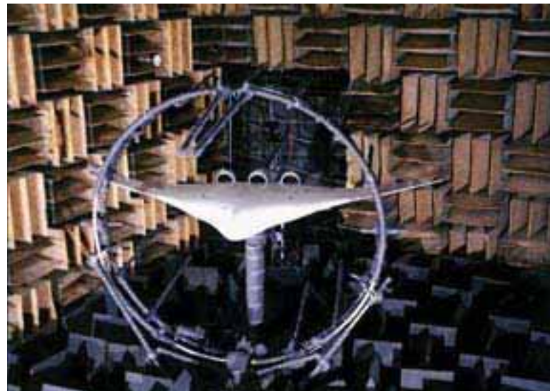
Acoustic tests of the BWB-800 configuration in the Langley Anechoic Noise Research Facility.
