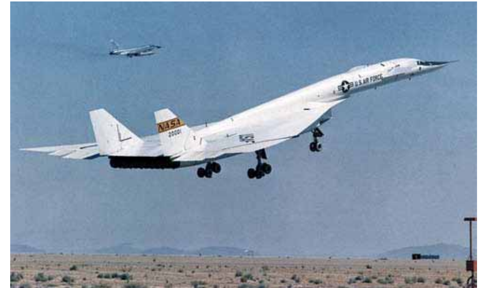
The XB-70 was used in NASA research on supersonic drag and sonic booms.
