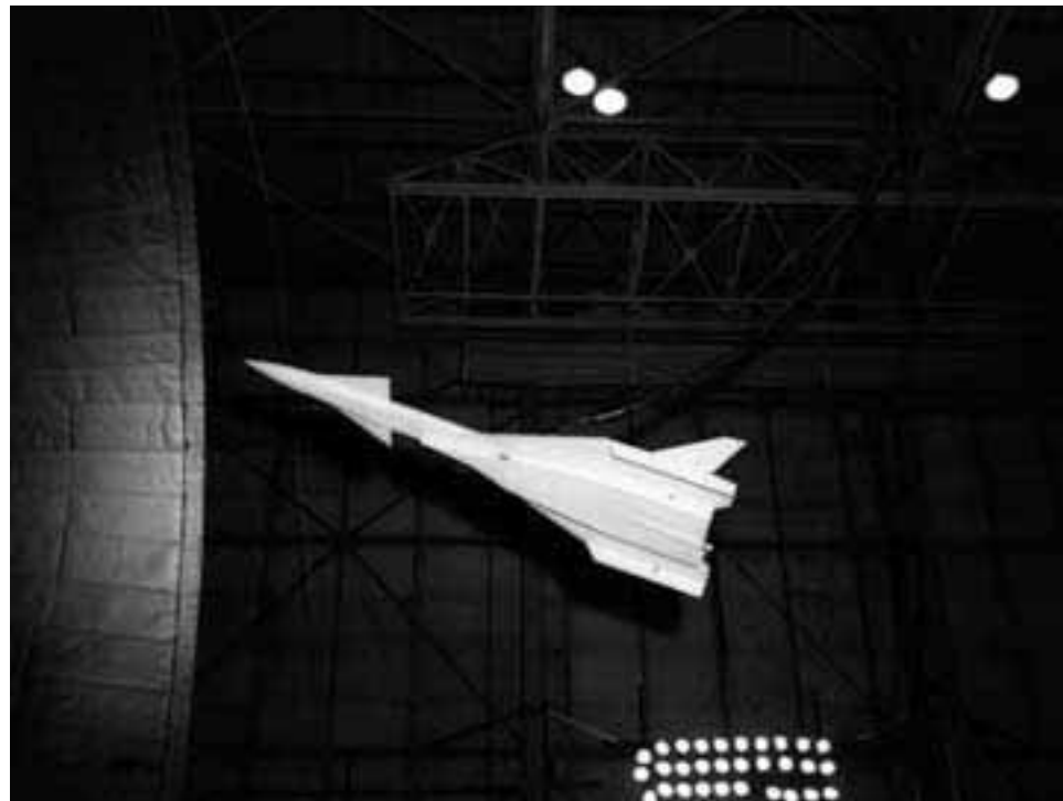
Free-flight model testing of the early XB-70 design was conducted in the 30- by 60-Foot Tunnel in 1957.
