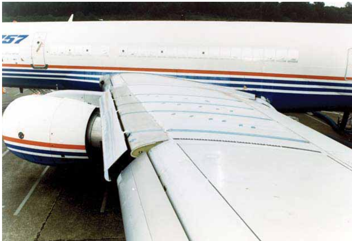
View of the instrumented left wing of the 757 test aircraft showing the test panel area, hot-film gauges, pressure tubing, and the leading-edge Krueger flap/insect shield.
