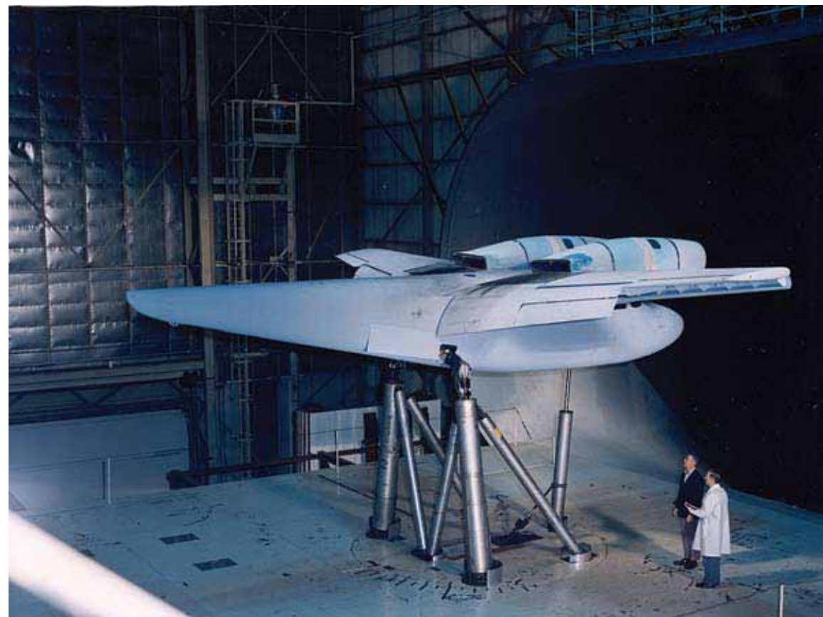
Langley researcher Charles C. Smith, Jr., and technician Charles Schrum inspect the modified Aero Commander USB research model in the Langley Full-Scale Tunnel.
