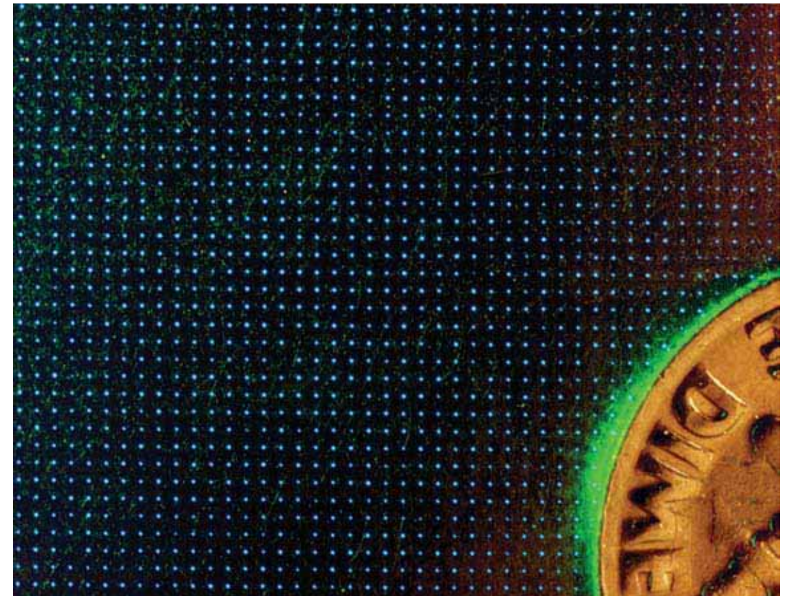
Size of holes in F-16XL test glove compared with a dime.
