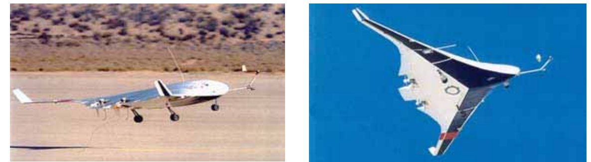
The 6-percent remotely controlled blended wing body model flown by the Stanford University Advanced Concepts for Aeronautics Program team.
