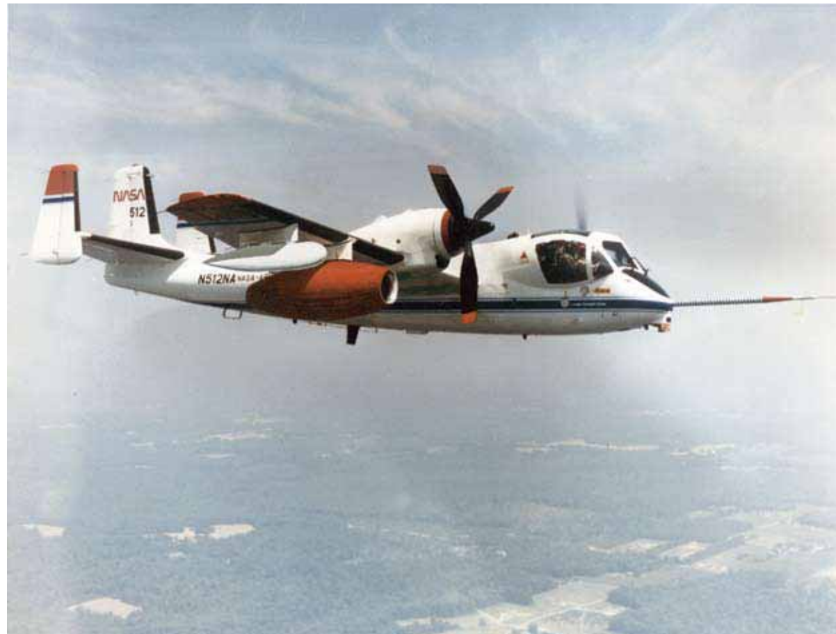
The NASA OV-10B in flight with an NLF nacelle under the right wing. Note feathered propeller and underwing pod containing noise source.
