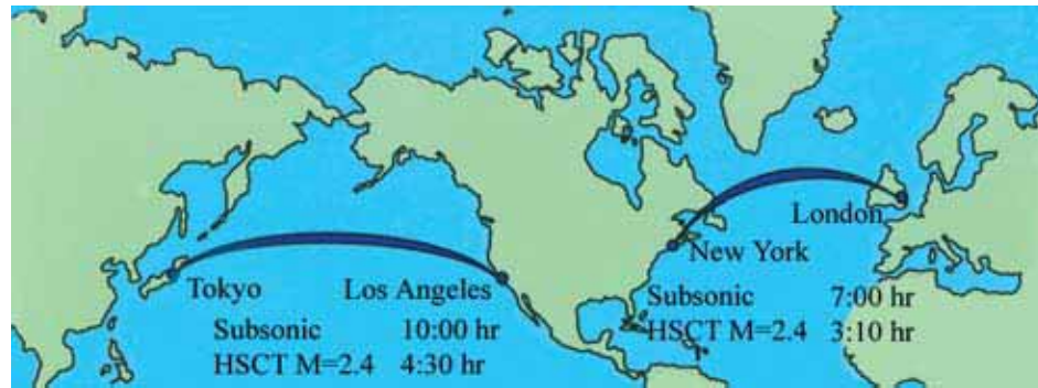
Comparison of international travel times for a conventional subsonic transport and an advanced Mach 2.4 high-speed civil transport.
