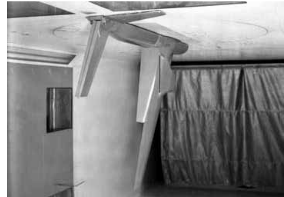
Model configuration used in early Langley USB research in 1957 mounted to the ceiling of the Langley 300-mph, 7- by 10-Foot Tunnel.
