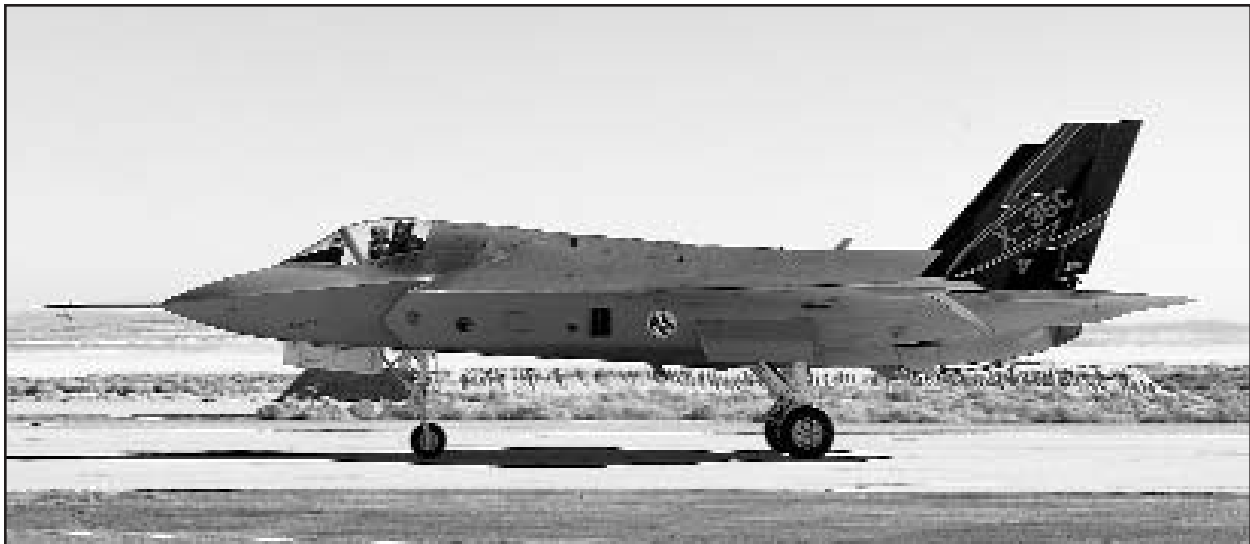
The X-35C demonstrator taxis at Palmdale prior to its first flight. Note the faceted intakes on the side of the fuselage and the colorful tail markings unique to the X-35C. (Lockheed Martin via the Tony Landis Collection)
