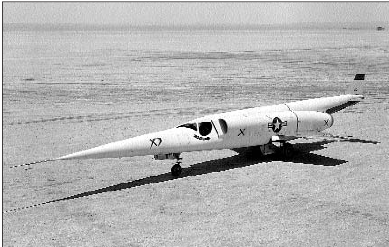
The X-3 was designed to explore high speed aerodynamic phenomenon at speeds of Mach 2 for half an hour. Unfortunately, a lack of suitable engines ultimately doomed the aircraft as a research tool. (NASA photo E-2412)
