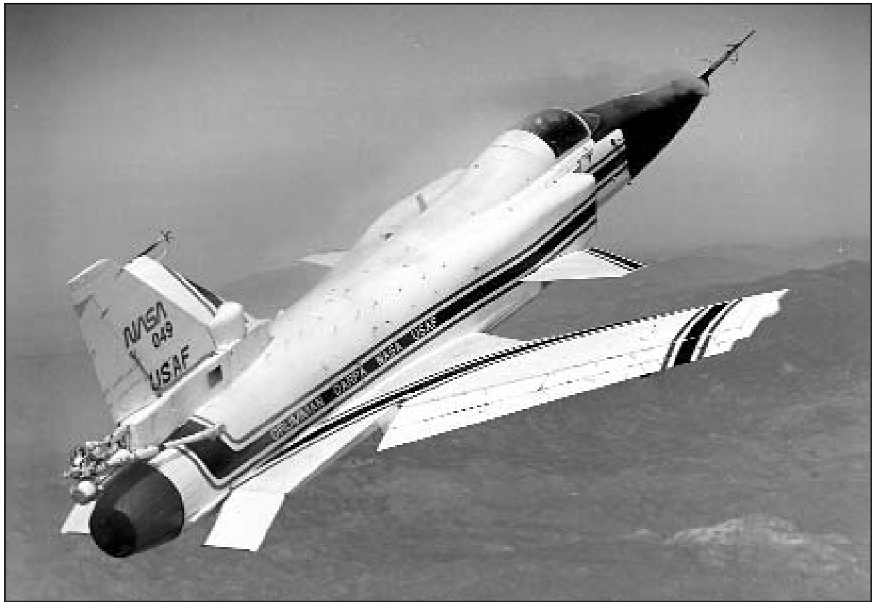
The X-29A proved many of the advantages of the forward swept wing, but also showed that the configuration generated a great deal more drag in some flight regimes than expected. (NASA photo EC91 491-7)
