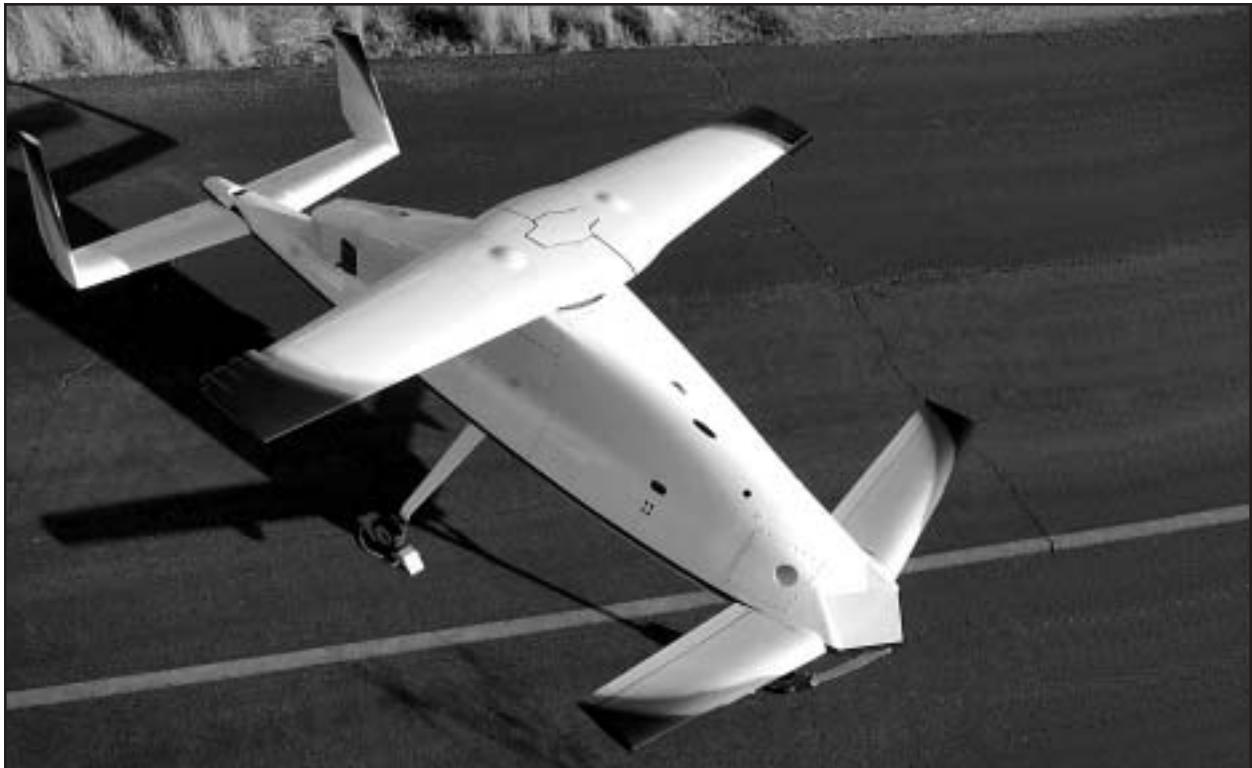
The Boeing Dragonfly demonstrator vehicle showing its centrally mounted rotary wing, its movable forward canards, and its fixed horizontal stabilizer. (Boeing via Erik Simonsen)
