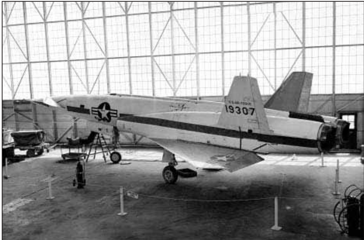
The X-10 was an aerodynamic and systems testbed for the MX-770 (B/SM-64) Navaho Mach 3 intercontinental cruise missile. A total of 13 X-10s were manufactured, although only 10 were flown. (The Boeing Company Archives)
