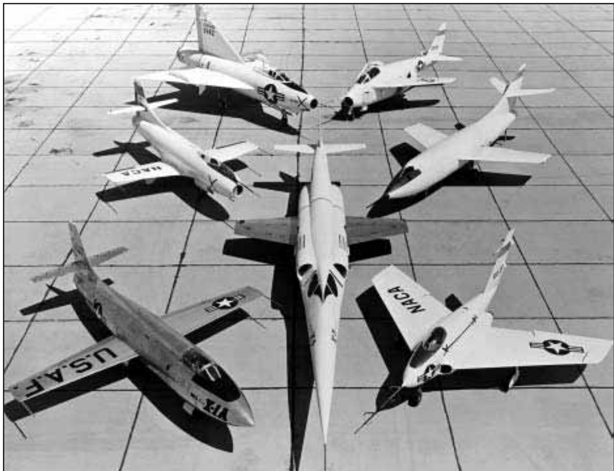
The experimental aircraft fleet at the Flight Research Center in 1957. Clockwise from left front: X-1A, D-558-I, XF-92A, X-5, D-558-II, X-4, and the X-3 in the center. (NASA photo E-2889)
