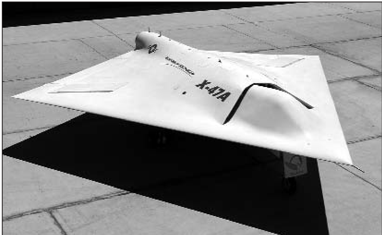
The overall shape of the X-47A is very reminiscent of the "hopeless diamond" originally conceived during the development of the F-117 stealth fighter. Note the complete lack of vertical control surfaces. (Northrop Grumman)
