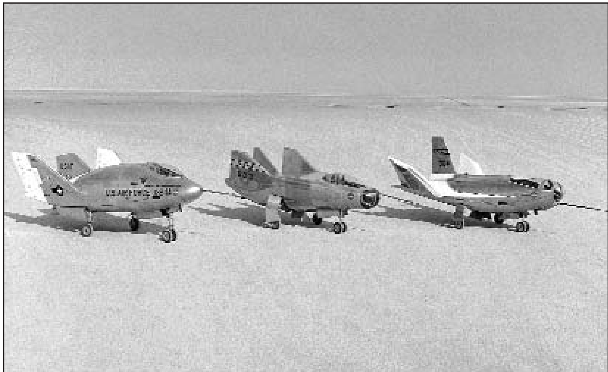
The three lifting bodies tested during the 1960s: The Air Force X-24 (described separately) is at left, the M2-F3 is in the center, and the HL-10 is at right. All proved to be remarkably capable machines, especially given the limited budget used for their development.
