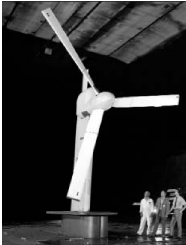
Figure 26. Boeing 26-ft. diameter proprotor on semi-span wing in the Ames Research Center 40- by 80-ft. wind tunnel. (Ames Photograph AC72-5255)
