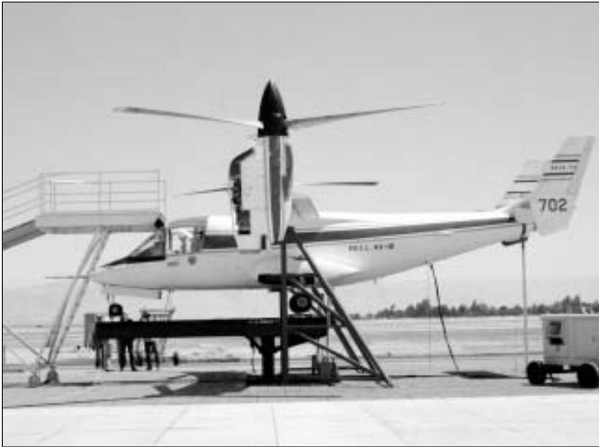
Figure 49. Tiedown test facility at the Ames Research Center showing the hydraulic lift. (Ames Photograph AC80-0686-3)
