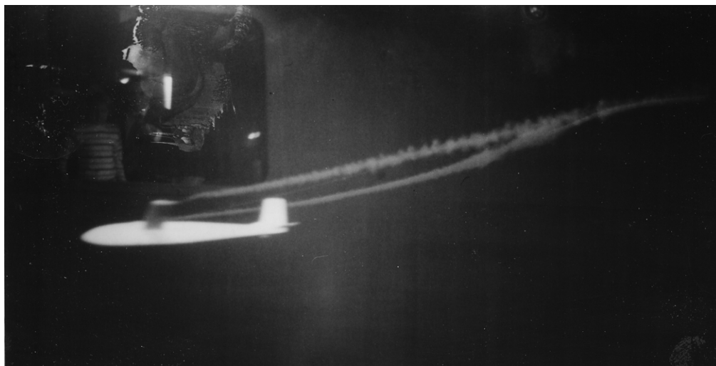
FIGURE 7.5. Heavily weighted glider (40-in. wingspan) gliding slowly (about 3 ft/s) underwater in large tank. Fluorescent dye is emitted from wing tips. When glider made complete circles, trails from previous circle were always well above glider.
