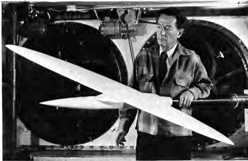
May 22: Dr. Robert T. Jones of Ames Research Center stood by the wind-tunnel model of a conceptual aircraft being developed in computer and wind-tunnel studies. The fan jet transport's wing would rotate 45^\circ or more above a center pivot as the speed increased, in attempt to achieve supersonic speed without high fuel consumption and noise. By taking off with the wing perpendicular to the fuselage, the aircraft would require one fourth the takeoff energy of comparable delta-wing transports.
