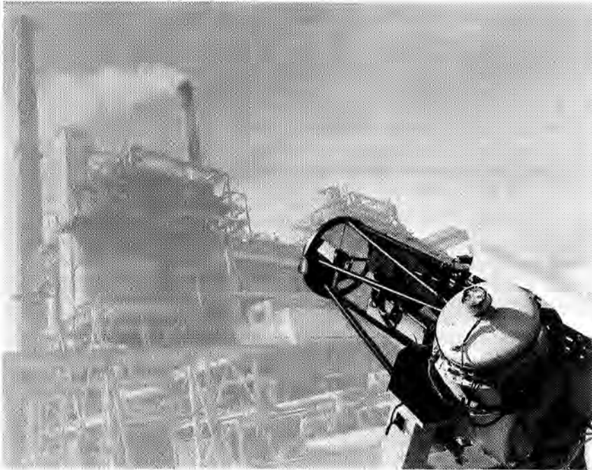
November 21: A telescope-mounted laser instrument was beamed at exhaust stacks of an industrial plant in tests proving the laser's ability to detect such air pollutants as sulfur dioxide. Remote detection from as far as one kilometer (3300 feet) was possible by the laser, developed at Langley Research Center. Tests were being conducted at the Carolina Power and Light Co. plant in Asheville, N.C., which had offered to cooperate in the LARC and Environmental Protection Agency program.
