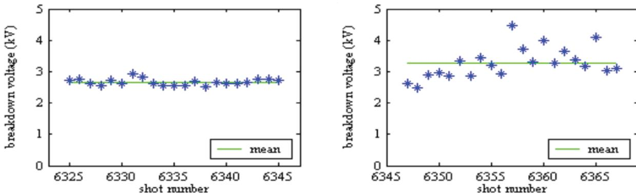
Figure 5. (Left) Example slow-rising, low-energy, DC breakdown voltages for multiple insulation samples. The samples broke down at an average of  $2.8 \pm 0.2$  kV. (Right) When exposed to slowly rising DC after the application of the PASD pulse, the average breakdown voltages remained the same or actually increased. This is a common high-voltage conditioning phenomenon.
