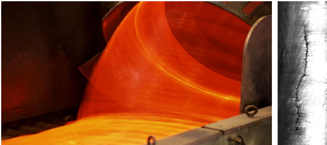
Figure 16: Left: Steel being coiled; Right: A 900 mm by 3 mm "seam" detected by the HotEye™ system.
