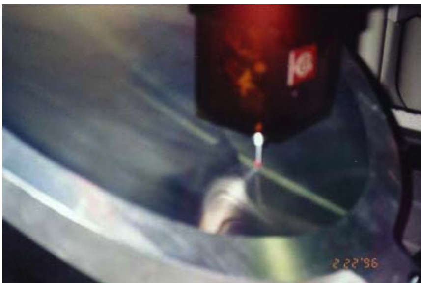
Figure 14: Plasma beam cleaning and polishing the surface of a wafer. (Image: Courtesy of RAPT Industries)
