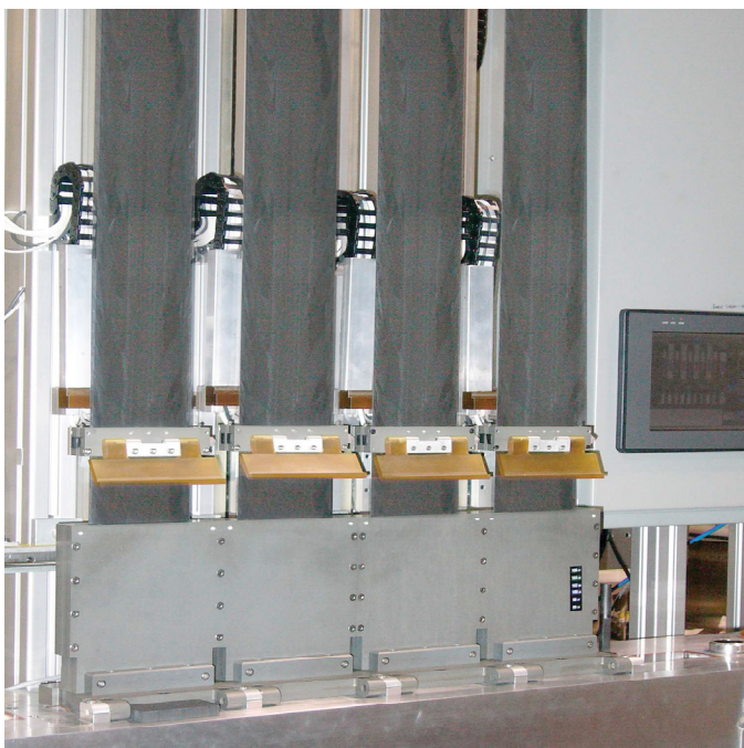
Figure 19: Left: Four silicon wafer pulling machines; Right: A pair of “strings” pulling silicon from a crucible. (Images: Courtesy of Evergreen Solar, Inc.)
