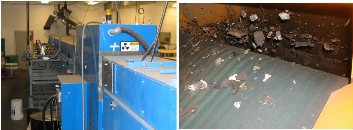
Figure 10: Left: The Spectramet® alloy sorter consisting of a sorting chamber and material ejectors; Right: Non-ferrous metals tend to be ejected farther than non-metals (plastics, rubber) and thus can be separated by a splitter plate prior to being sorted by the Spectramet® alloy sorter.
