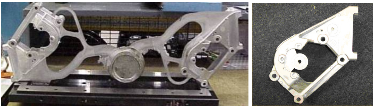
Figure 9: Left: Two components cast conventionally illustrating offal (biscuits, runners, flash); Right: Single component “as cast” via the new technology. (Images: Courtesy of Ford Motor Company)
