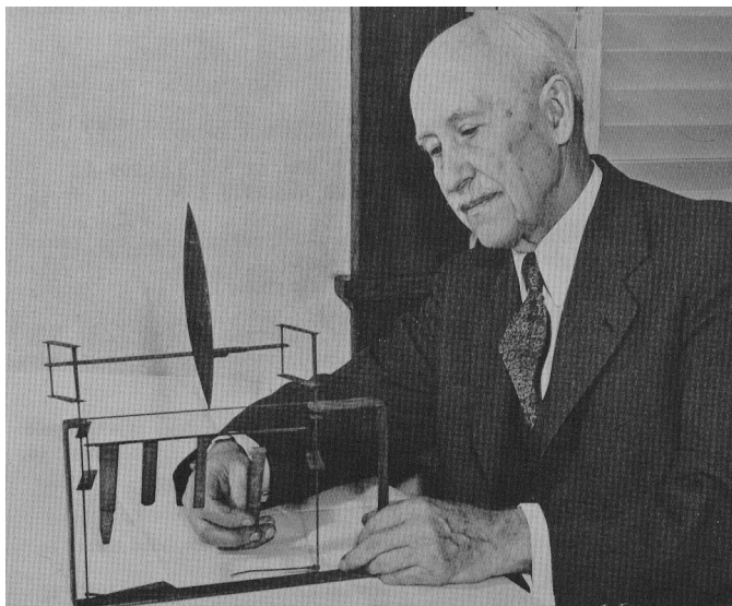
Orville in his laboratory at 15 North Broadway, Dayton, in December 1946, with a wind tunnel balance constructed in 1901.
