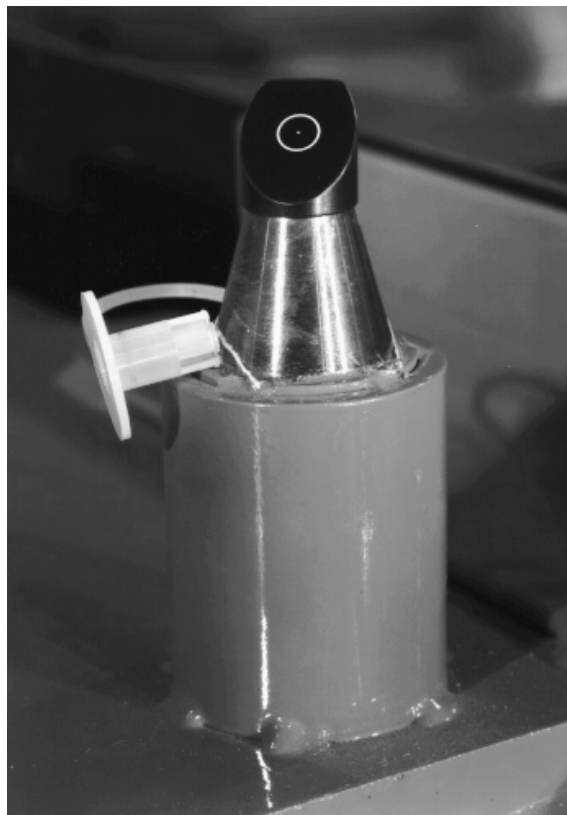
Figure 2. Fiducials accept a tooling ball or an optical target (above) for direct sighting with survey instruments.
