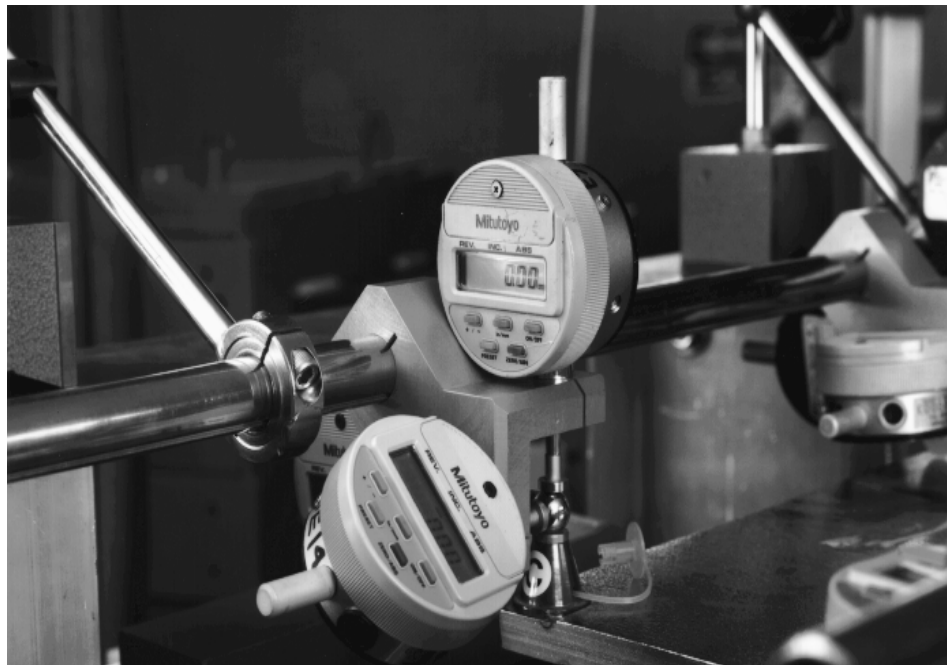
Figure 1. Fiducials must be configured to accept a tooling ball.
