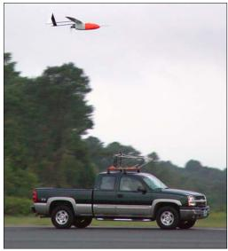
An aerosonde unmanned aircraft being released from its transport vehicle on the runway at the NASA Wallops Flight Facility, in Wallops Island, Virginia, on September 16, 2005.
