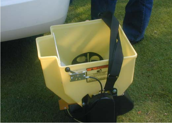
Manually Operated Native Grass Drill
