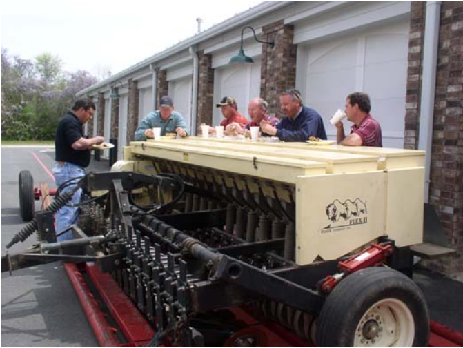
Grass Drill Designed to Plant Native Grasses Demonstrated at Training
