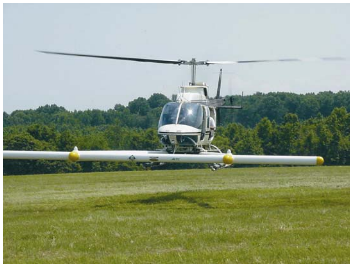
Figure 3c. MTADS Kit on Helicopter
