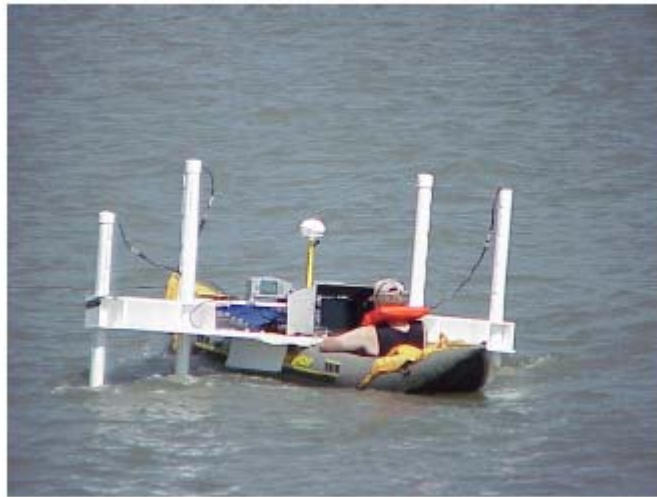
Photo 6. Geophex's deployed Geonics 858 Magnetometer System.
