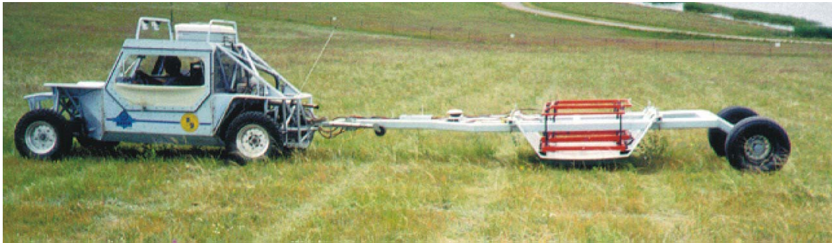
Figure D-11. EMI Array
