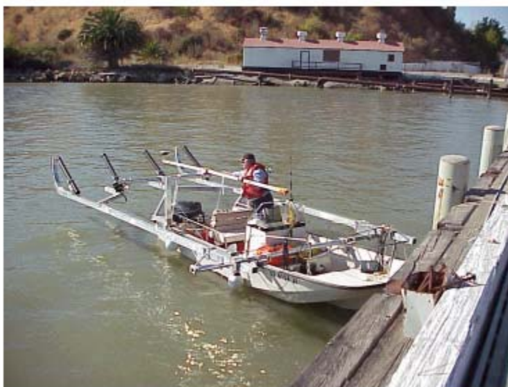
Photo 5. Alpha Geoscience/SONTEC mounted AGS-2 Magnetometer.
