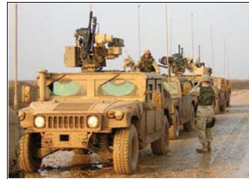
Common Remotely Operated Weapon System-equipped humvees navigate a road in Iraq last year. The new system's advanced technology provides 98 percent accuracy.
