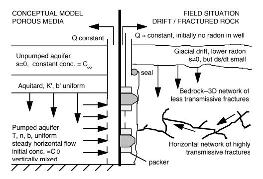
Figure 1. Schematic of conceptual model for development of analytical and numerical solutions (left), and schematic of field situation in glacial drift / fractured rock system with vertically variable radon concentration (right).
