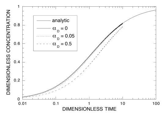
Figure 4. Dimensionless concentration versus dimensionless time for analytic solution with no dispersion, and for MOC3D solutions with dimensionless dispersivities of 0, 0.05, and 0.5.
