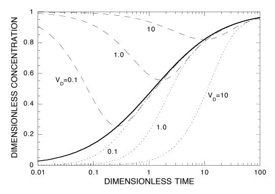
Figure 2. Dimensionless concentration versus dimensionless time for flow entering the well (C<sub>D</sub>, solid) and for pump discharge (C<sub>pD</sub>, dashes and dots) for three dimensionless casing volumes. Dotted lines are for C<sub>p0</sub>=C<sub>0</sub> and dashed lines are for C<sub>p0</sub>=C<sub> $\infty$ </sub>.
