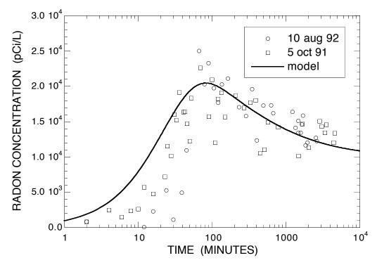
Figure 3. Illustrative calibration of analytical model with mixing in well casing to radon concentrations during constant-rate pumping tests on 5 Oct 91 and 10 Aug 92 in Mirror Lake area, Grafton County, New Hampshire.
