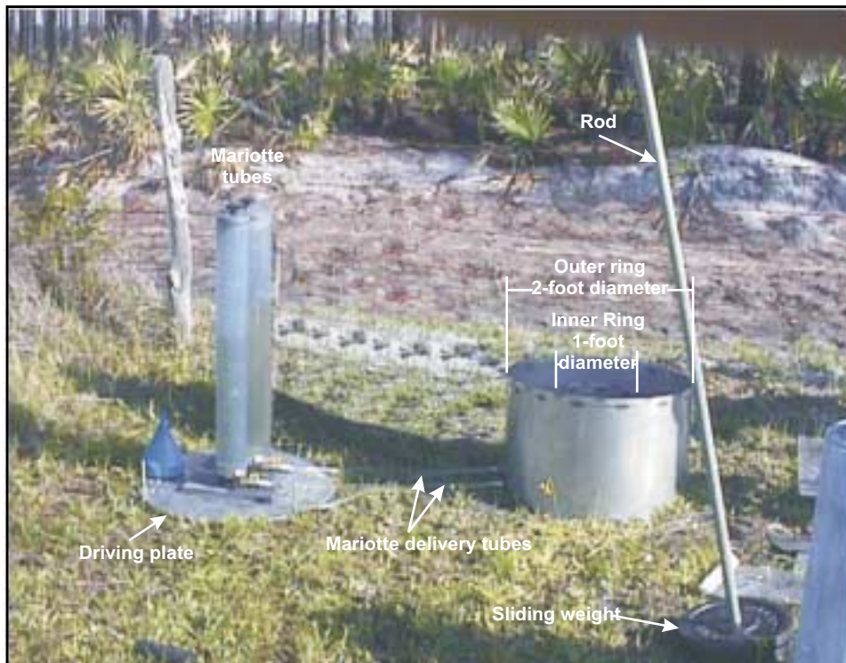
Figure 2. Double-ring infiltrometer setup.
