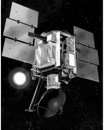
antenna with two spot beams that sweep in a circular pattern. The antenna radiates microwave pulses at a frequency of 13.4 gigahertz across broad regions on Earth's surface. The instrument will collect data over ocean, land, and ice in a continuous, 1,800-kilometerwide band, making approximately 400,000 measurements per day.
