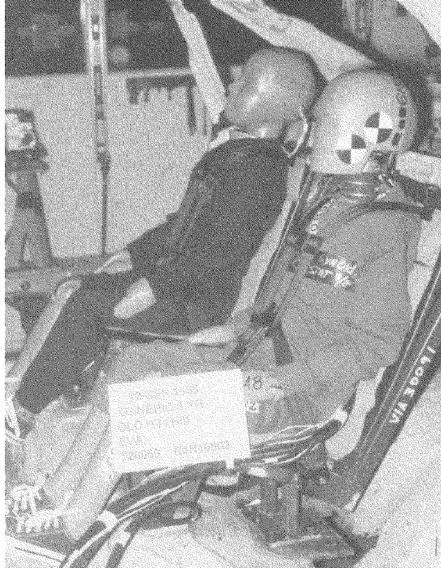
Figure 15 --Six-year-old dummies in rigid seat with 5-pt harness in Ford evaluation tests
