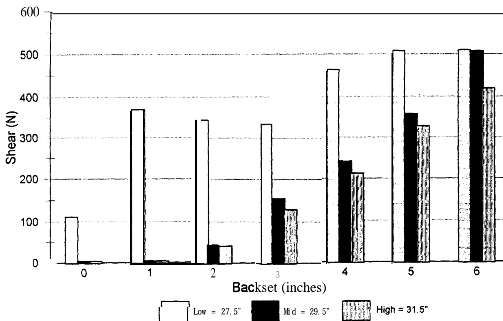
Figure 8: Maximum Positive Shear Force at the Occipital Condyles. The erratic trends in the shear forces at the low height are a result of the precise details of the rotation of the head over the head restraint and the location of the point of contact. At the intermediate and high heights, an increase in the backset caused delayed contact of the head with the head restraint and an increase in the peak shear forces.
