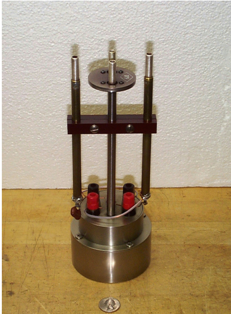
Fig. 17. A 10 pF fused-silica capacitance standard.
