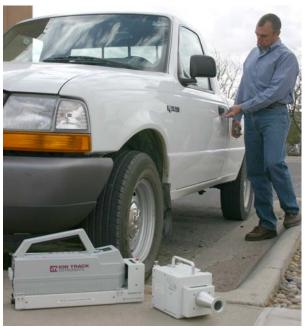
The Hound™ sample collection and preconcentration unit works with a commercial detector to detect trace explosives. The operator collects a swipe sample from a vehicle.
