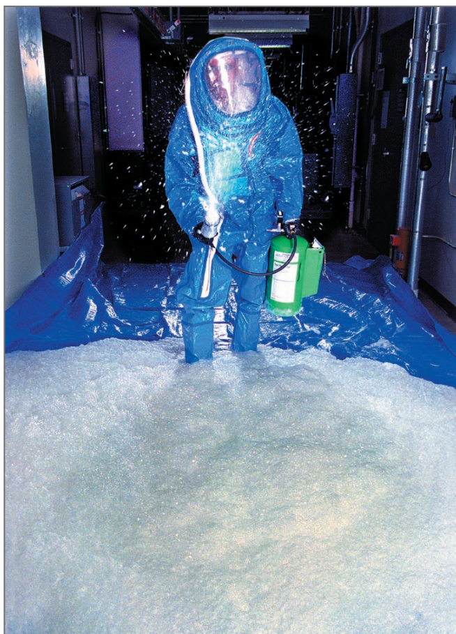
Foam developed by Sandia and now licensed to two commercial vendors was used to remediate portions of the Capitol Hill office buildings and news facilities in New York City.
