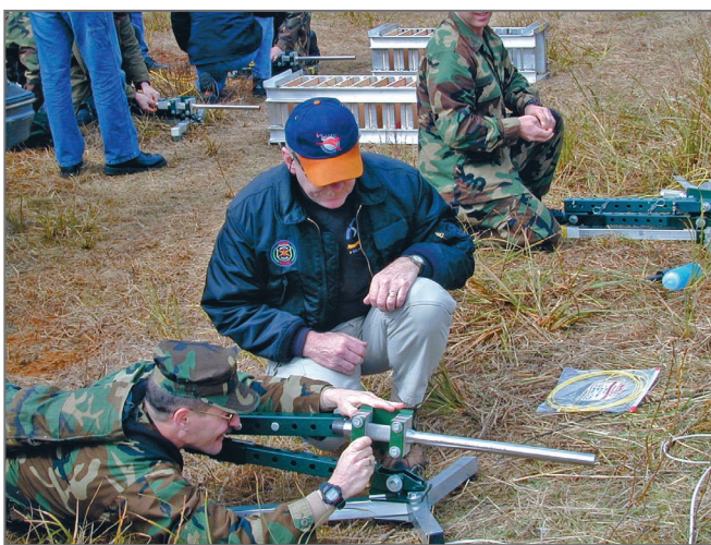
Bomb squad personnel learn to use Sandia's Percussion-actuated Nonelectric (PAN ® ) Disrupter at Operation America.
