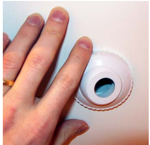
Puffs of air from nozzles dislodge explosives particles from a person's hair, skin, and clothing
