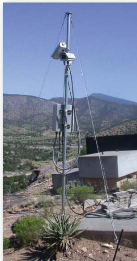
Cluster nodes gather data from sensor nodes and use cameras to survey the area.
