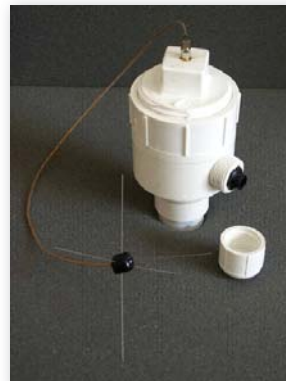
A VPED sensor node with an inconspicuous, ground mounted antenna gathers data from a variety of sensors and processes information for the cluster node.
