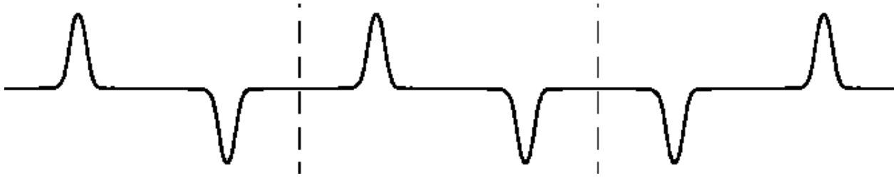
Figure 1.10 Gaussian doublet with delay between positive and negative pulses (ref. 11).
