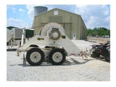
The TSE model 6811 reel winder is designed to handle the pulling rope or pulling cable when used with the TSE model P210-1H/1DD bullwheel puller.
