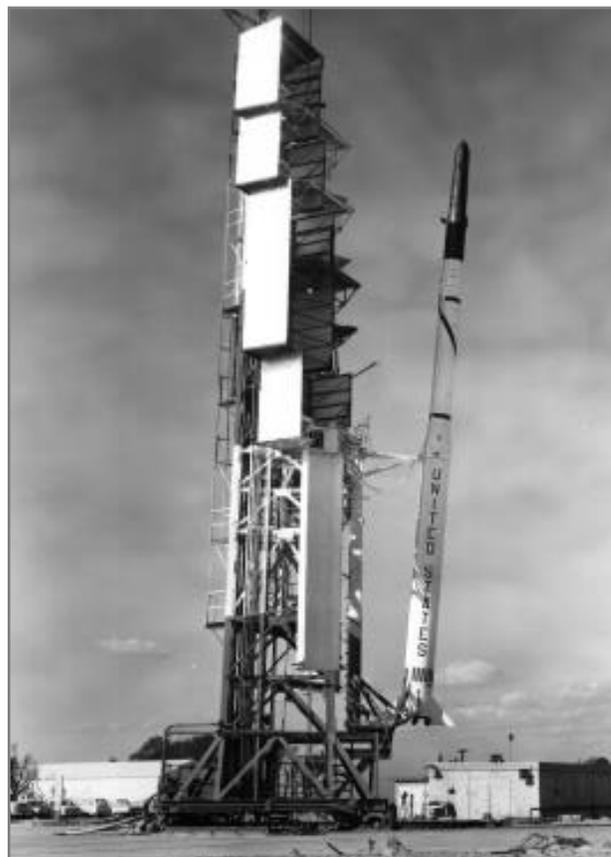
The Scout launch vehicle is shown ready for launching in 1962 at NASA’s Wallops Station (now called the Wallops Flight Facility). Scout was a four-stage, solid-fueled vehicle that stood 72 feet high and weighed about 36,100 pounds.
