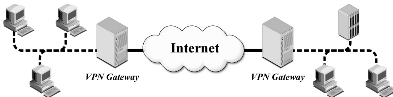
Figure 2-2. Gateway-to-Gateway Architecture Example
