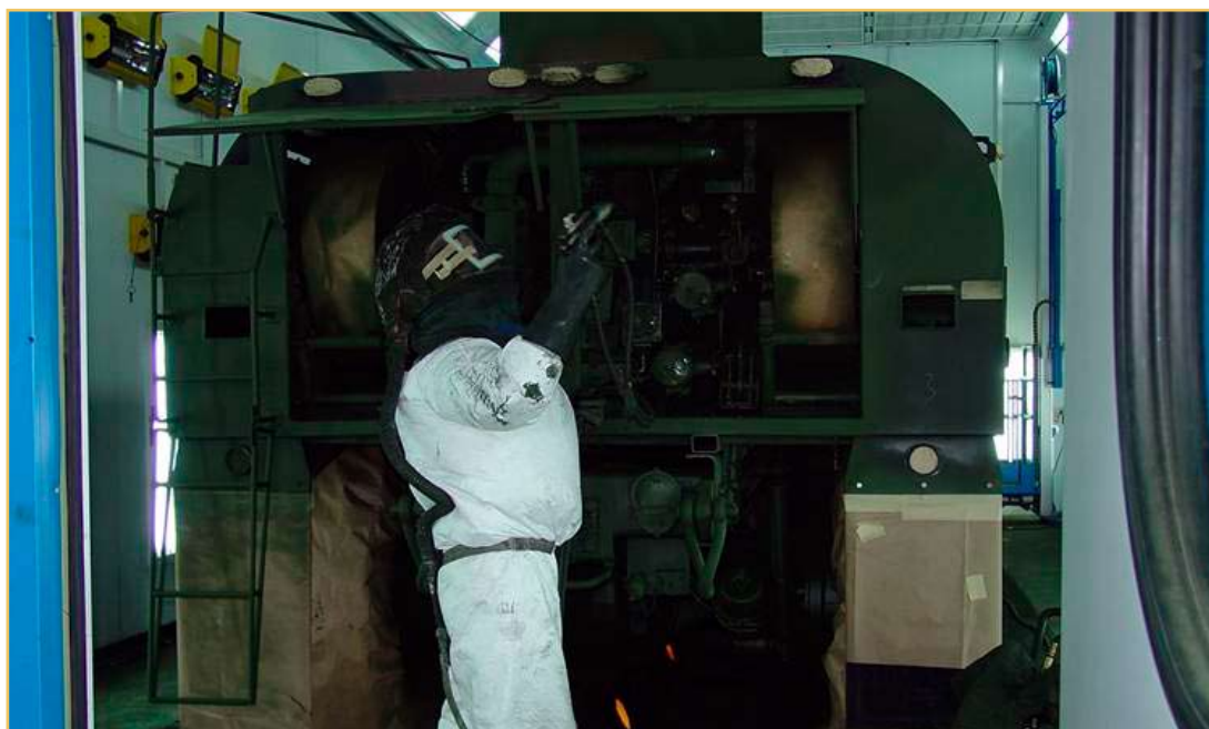
US Army Material Support Center Korea Korean National employee uses the new water-based CARC paint application system.
