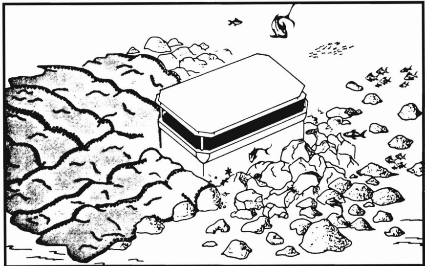
Figure 6.—Artist's rendition of the experimental tarpaulin partially covering the rock boulder (riprap) substratum surrounding the Redondo Beach Units 7 & 8 intake structure. (From Helvey et al., 1981.)
