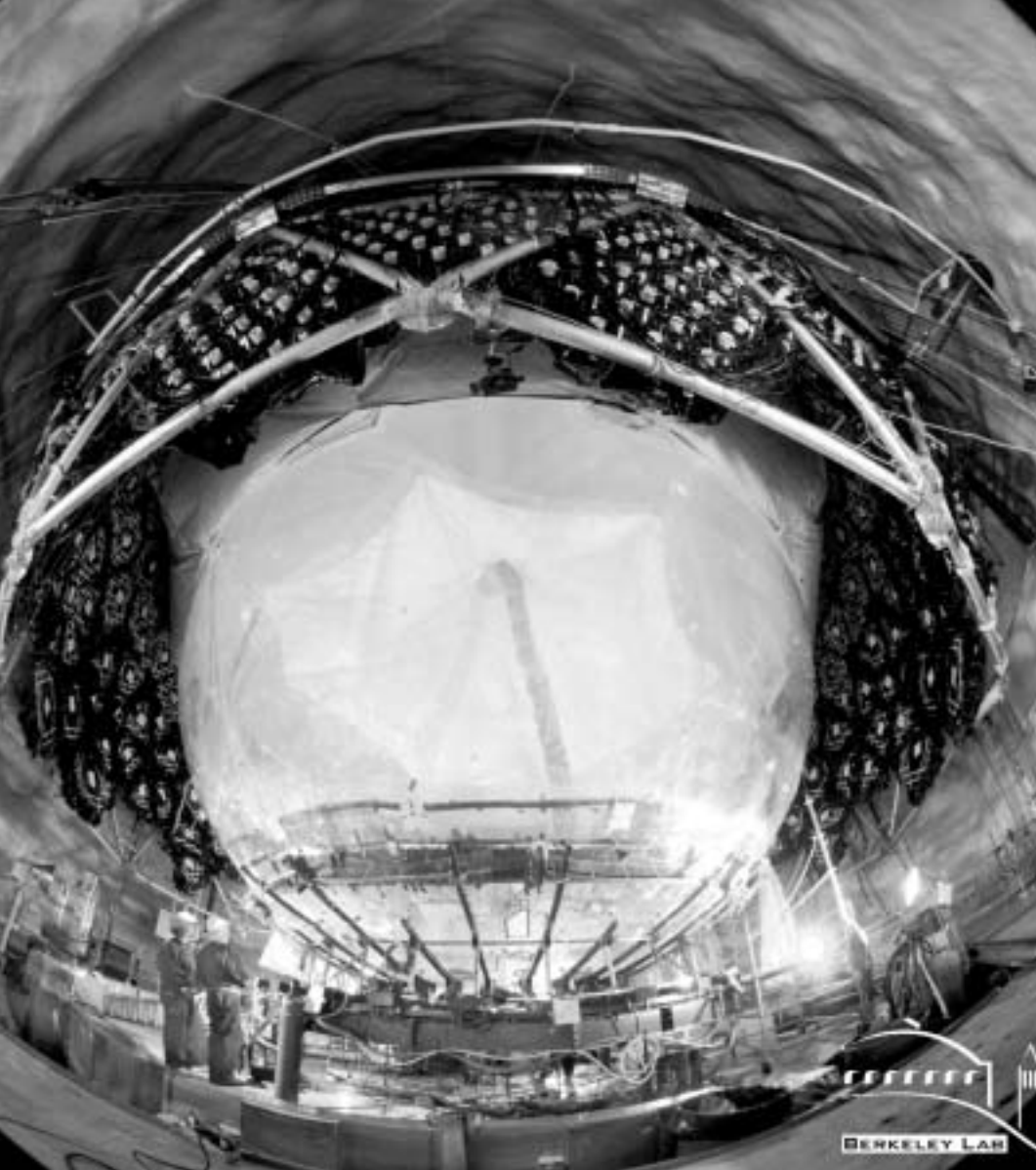
The SNO detector just before completion of the bottom of the acrylic vessel. The acrylic used for this vessel is over 2.5 inches thick and built to hold 1000 tons of heavy water.
