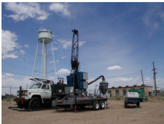
Drill rig used to obtain samples of melt material
