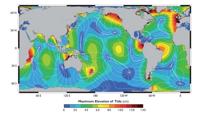
The tide is composed of multiple waves, the largest of which is denoted M2, shown here as determined by TOPEX/Poseidon measurements. This M2 wave cycles once in half a lunar day, or about every 12.4 hours. Colors show maximum elevation at M2 high tide, in cm. White lines connect places that experience high tide simultaneously. To predict the full tide at any place, a dozen or more such waves must be added together.
