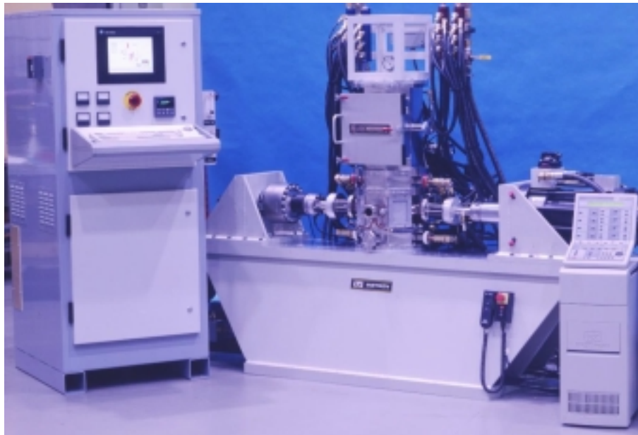
Fig. 3 Load frame and furnace attachment for SMARTS
