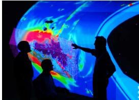
Researchers at Sandia's Visualization Laboratory discuss a computer simulation and analysis showing the impact of a foam piece along the leading edge of the space shuttle *Columbia's* wing.
