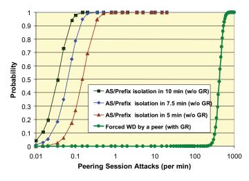
Fig. 12. Probability of adverse impact on routing as a function of peering session attack rate for BGP with/without GR (Q = 0.25, n = 4).
