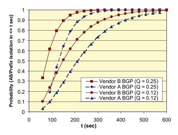
Fig. 8. Probability of AS-prefix isolation - Sensitivity to vendor parameters and probability of successful session attack (n = 4).
