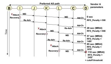
Fig. 3. Illustration of update message propagation and RFD penalty accumulation for the preferred AS path between nodes B and D.
