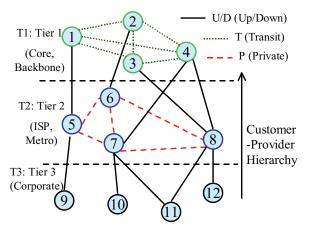
Fig. 20. Example AS-level network for policy illustration.
