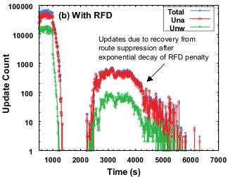
Fig. 15. BGP update count as a function of time: (a) vs. (b) comparison shows the suppression followed by flurry of updates after RFD penalty decays.
