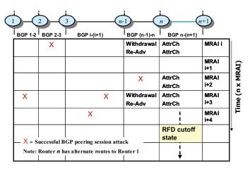
Fig. 6. Time-space model for relating RFD penalty accumulation to attacks and derivation of probability of successful AS-prefix isolation.
