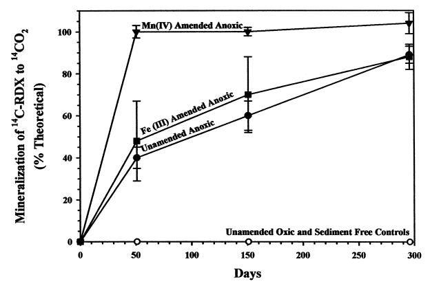
FIGURE 1 Effect of oxygen, Mn(IV), and Fe(III) amendment on mineralization of <sup>14</sup>C-RDX to <sup>14</sup>CO<sub>2</sub> in NSB Bangor sediment microcosms and sediment-free control microcosms. Unamended anoxic microcosms were Mn(IV)-reducing.
