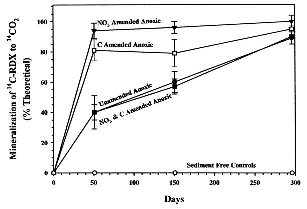
FIGURE 2 Effect of NO<sub>3</sub> and carbon (C) amendment on mineralization of <sup>14</sup>C-RDX to <sup>14</sup>CO<sub>2</sub> in NSB Bangor sediment microcosms and sediment-free control microcosms. Unamended anoxic microcosms were Mn(IV)-reducing.
