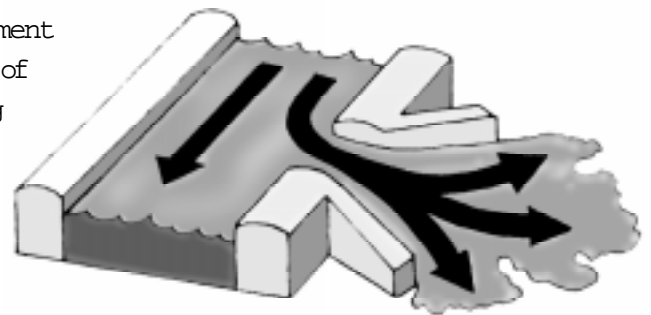
A cut in the levee allows fresh water and sediment to flow through and create new marshes.
