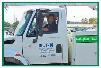
JERRY MURR GETS A FEEL FOR THE POWER OF A HYBRID BUCKET TRUCK. THIS TRUCK CAN OPERATE A BOOM ON ELECTRIC FOR TWO HOURS BEFORE RECHARGING ITSELF, SAVING **10-60%** ON DIESEL.
