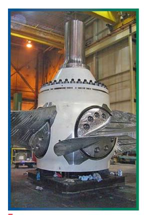
THE BEEFIER NEW RUNNER HUB IS DESIGNED TO WITHSTAND THE FORCES DELIVERED BY THE ARKANSAS RIVER ONCE IT IS INSTALLED AT OZARK DAM POWERHOUSE.
