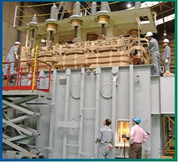
CARLOS VALENCIA (BLUE HELMET) OBSERVES AS Hyundai's engineers prepare to lower one of Norfork's new autotransformers into its tank.
