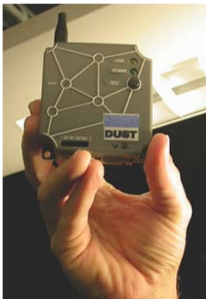
The Dust Networks mote shown here is part of a prototype lighting control system being tested to demonstrate wireless control of office fluorescent lighting for greater energy efficiency and occupant comfort.
