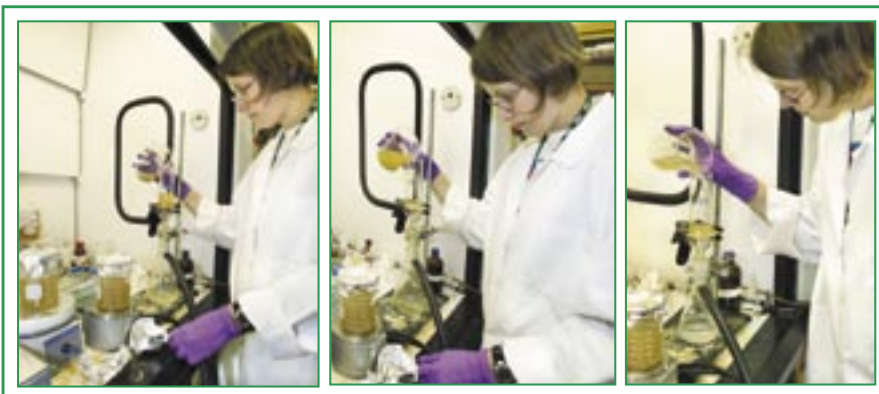
Figure 2. Researcher Christina Galitsky filters water after it has been mixed with the arsenic removal medium.
