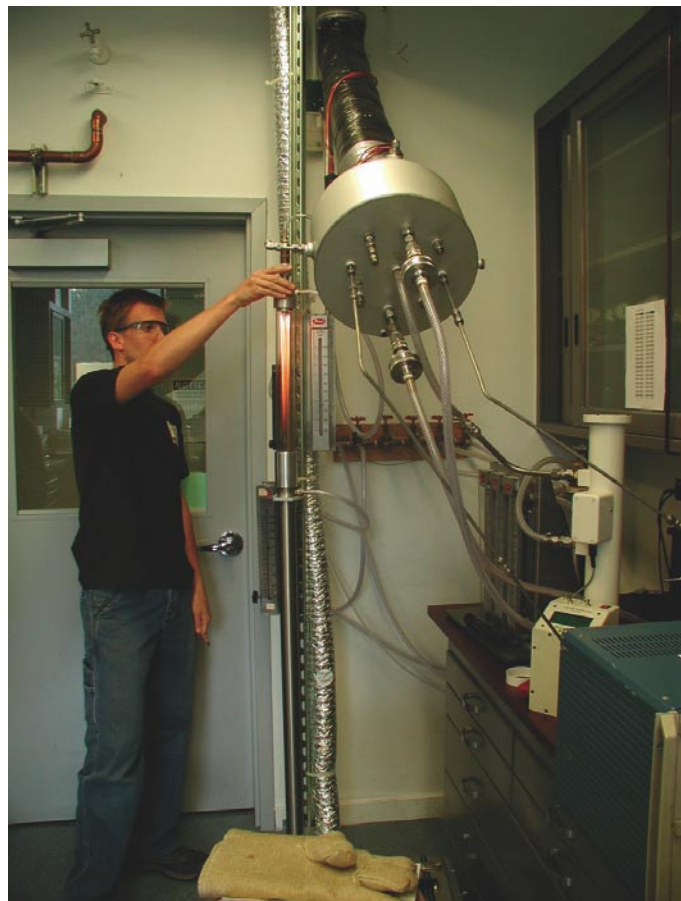
Figure 5. The multiple wavelength light transmission instrument (MULTI) (Photo credit Ted Gartner)
