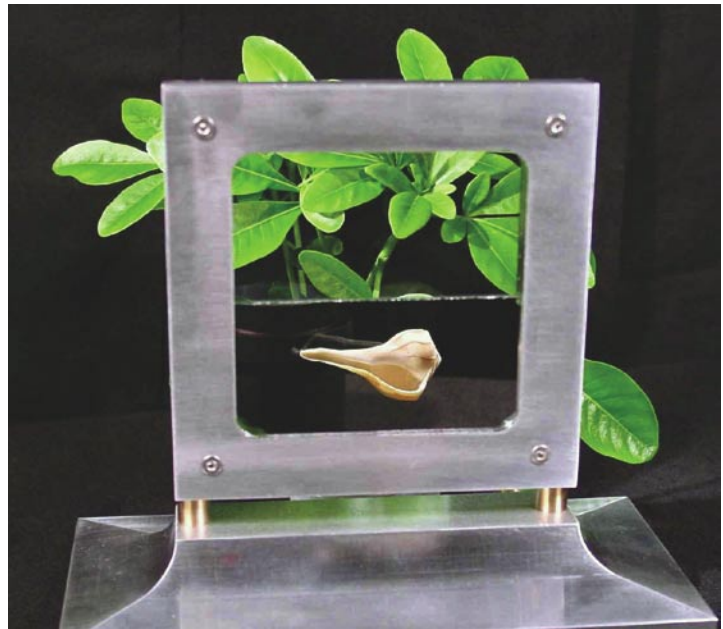
Figure 1. Transition-metal switchable mirror windows vary from transparency to heat and light (top half of this sample), to being almost wholly reflective (bottom)
