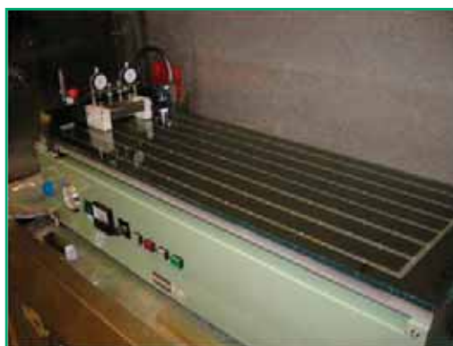
Figure 2. Electrode casting device.
