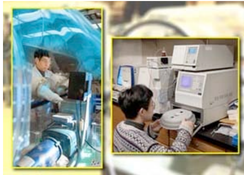
BATT FabLab researcher Gao Liu prepares a battery for testing. Inside a glove box, which controls water infiltration, he compresses the electrodes for higher energy density and better electronic contact (left). The test cells are finished in watch-sized, commercial form in the Klein machine (right).
