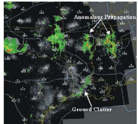
Figure 2 Anomalous Propagation & Ground Clutter
