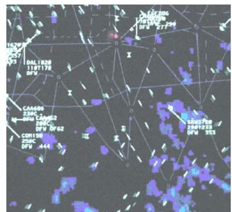
Figure 3 Air Traffic Controllers Display with NEXRAD Radar
