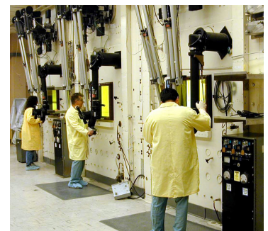
Los Alamos uses hot cells to develop remote nuclear fuel fabrication techniques and conduct advanced materials research.
