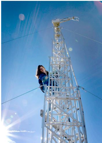
A Los Alamos scientist works on an eddy covariance tower used to measure CO 2 flux at the land-atmosphere interface.
